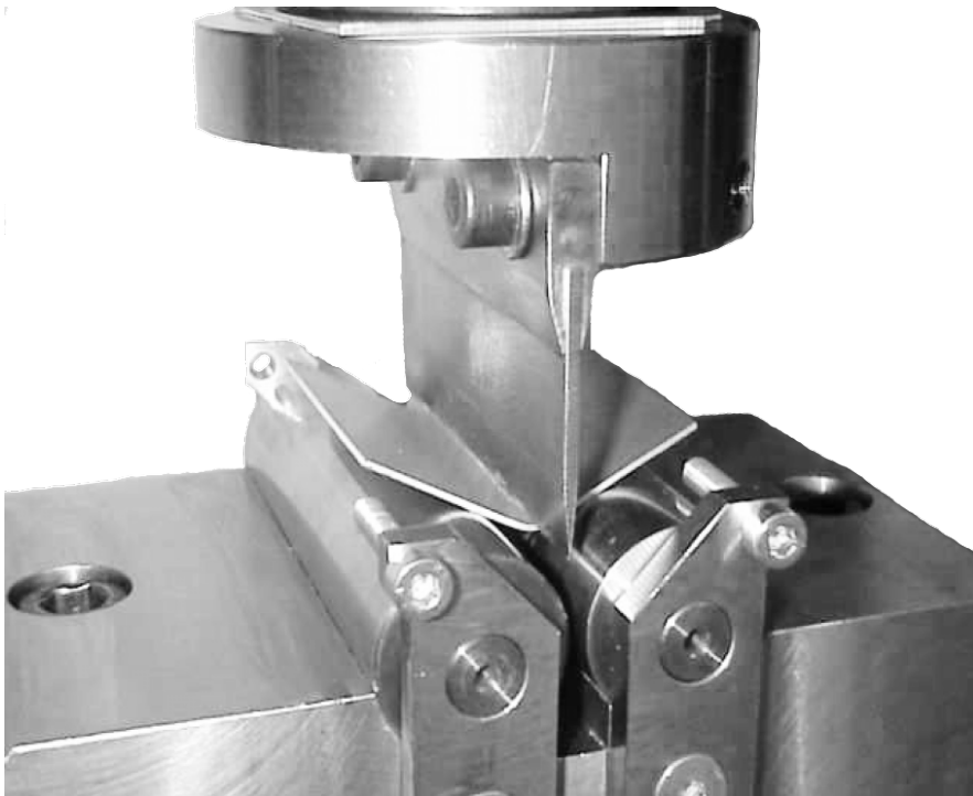
Hemming test – detection of crack strains
