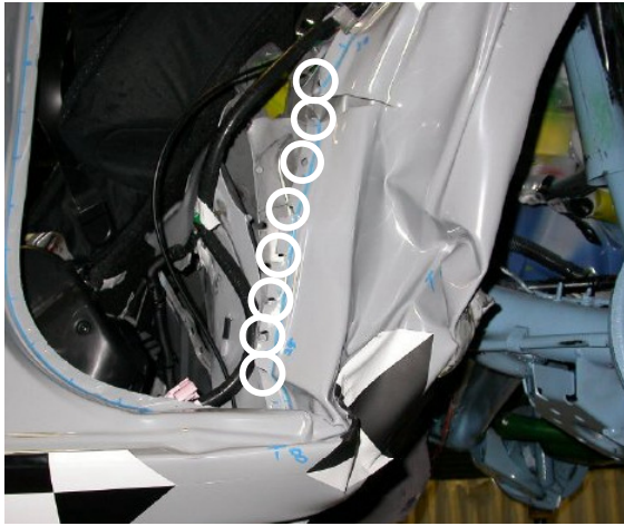
Fig 13: Ruptured spot welds in test (Left rear door opening)
