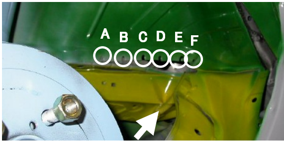
Fig 15: Ruptured spot welds in test (Right wheel housing)
