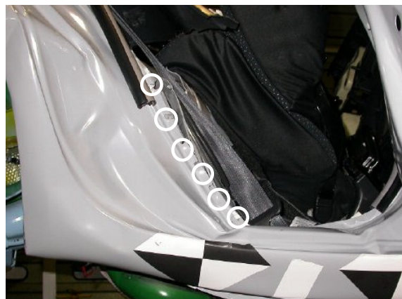
Fig 17: Ruptured spot welds in test (Right rear door opening)
