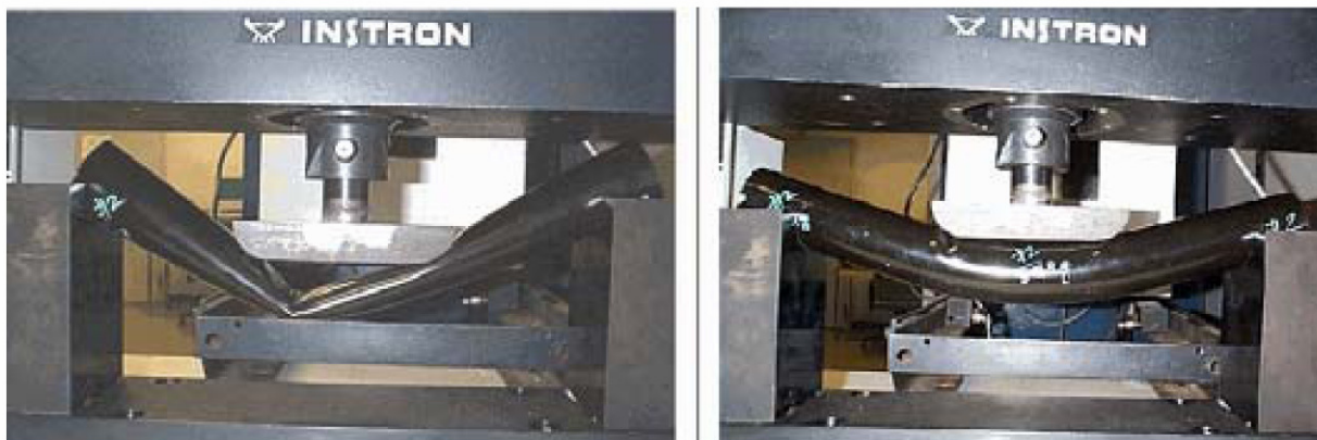
Figure 4: Load bearing capacity of an empty tube (left) and a foam filled tube (right)
