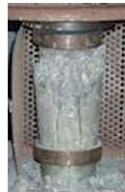
Concrete Cylinder Failure During Unconfined Compression Test By Courtesy of Schwer Engineering & Consulting Services
