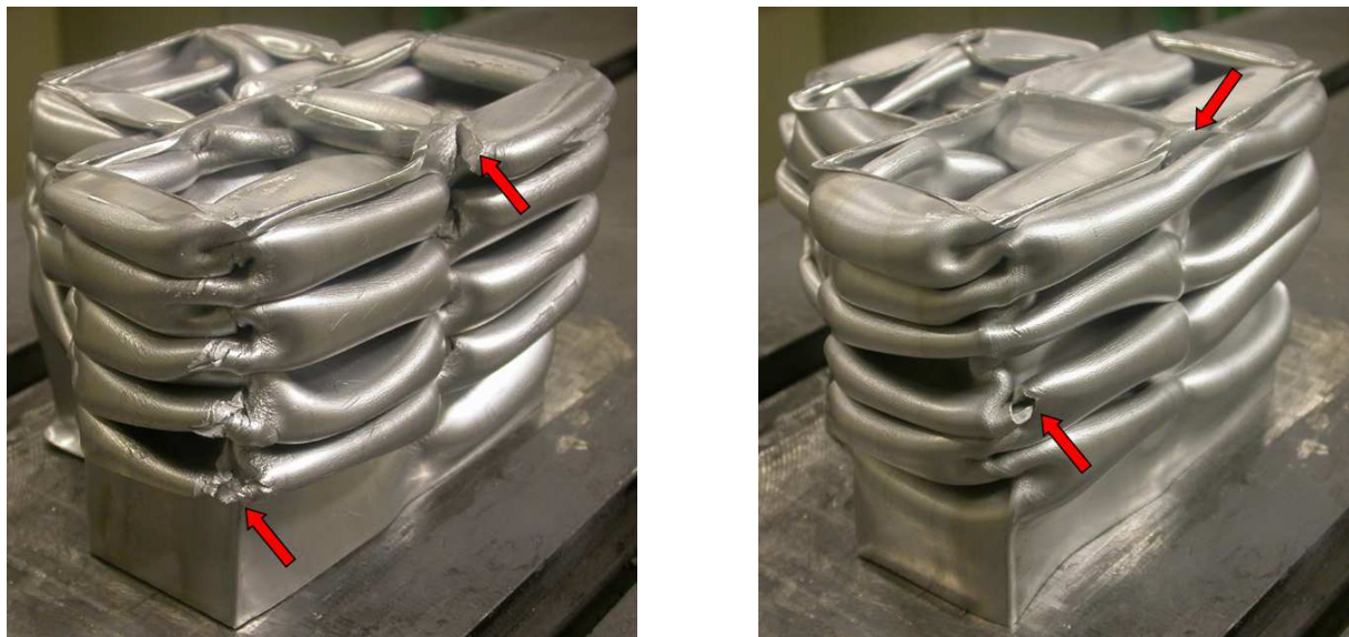
Fig. 1: Crushing tests with material variants that have the same yield stress
