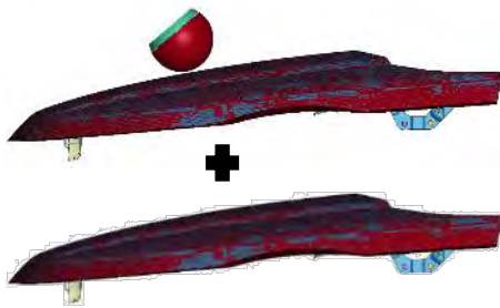
Hood optimization problem considering both impact and static load cases. Model courtesy of Jaguar Land Rover.
