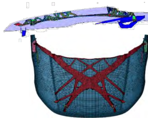
Final design of Hood with side view at upper and bottom view at lower
