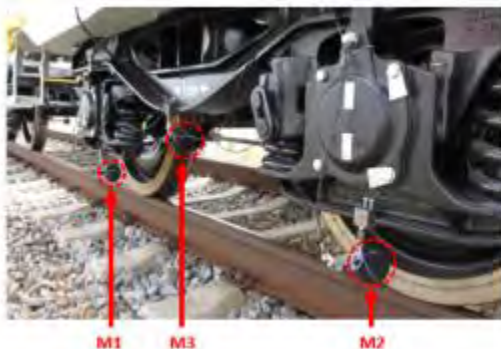
Experiment to evaluate pass-by noise levels at various speeds
