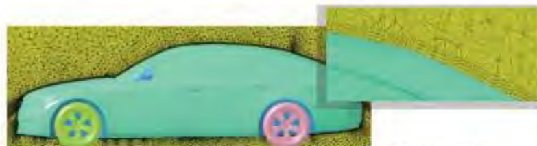
Fast mesh generation and automatic re-meshing with boundary layers
