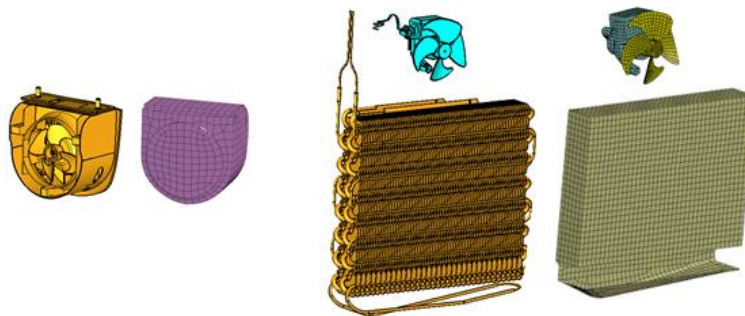
Fig.4: Example of geometry simplification on the evaporator fan system and the condenser coils
