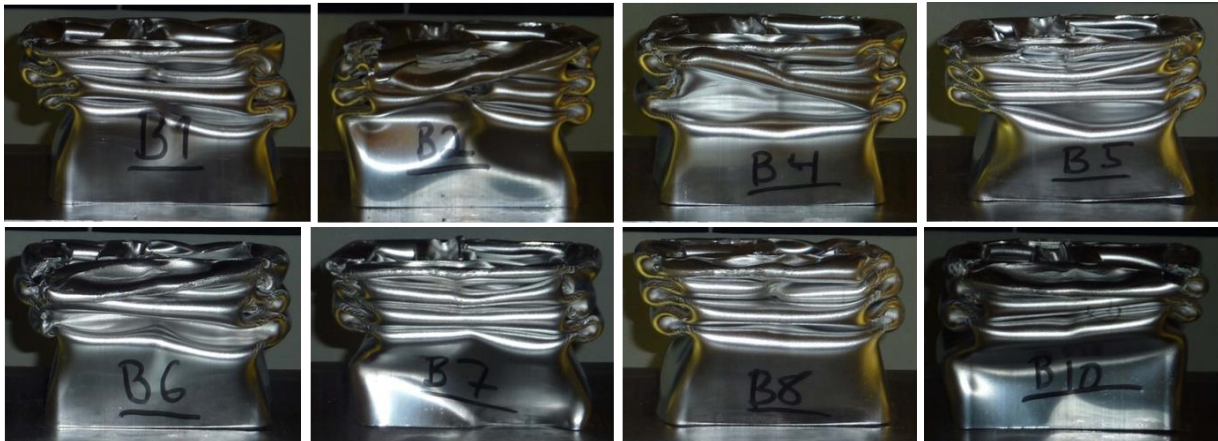
Fig. 1: Parallel tests show specimen 2, 4 and 6 that does not follow progressive folding.
