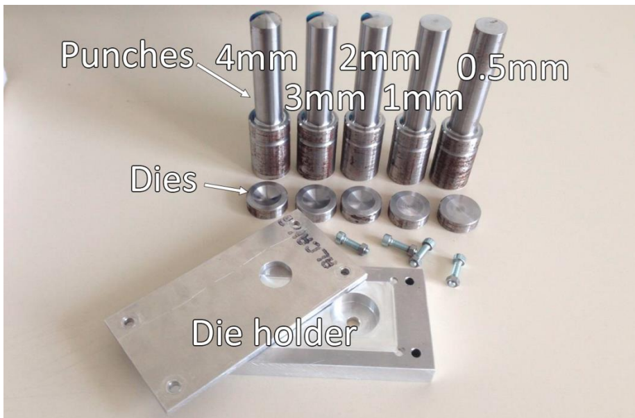
Fig.4: Components of the device for cold forming of sheet metal specimen [7].
