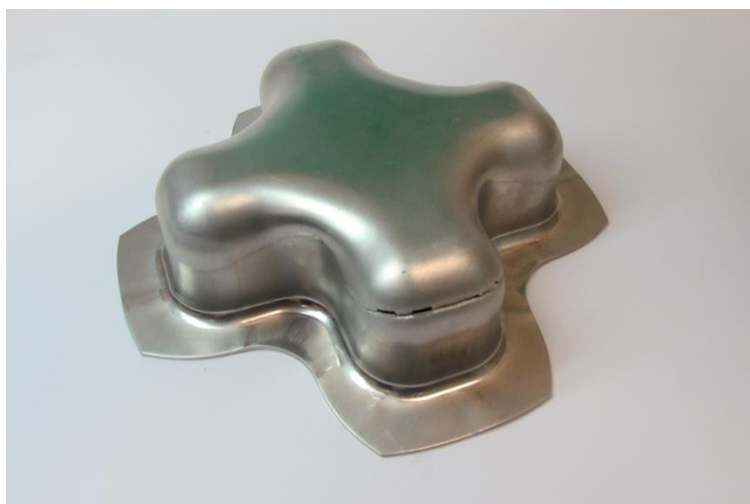
Fig.13: Cross-die specimen just after rupture. The maximum drawing depth of 53.6 mm was determined in successive trials with constant blank holder force.
