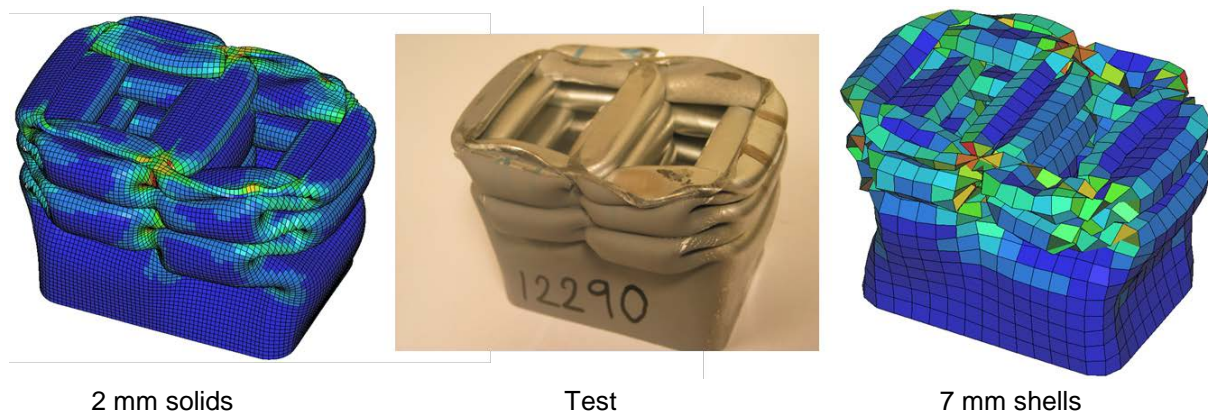
Fig.2: Predicted deformation mode with shell- and solid elements compared with the test result.
