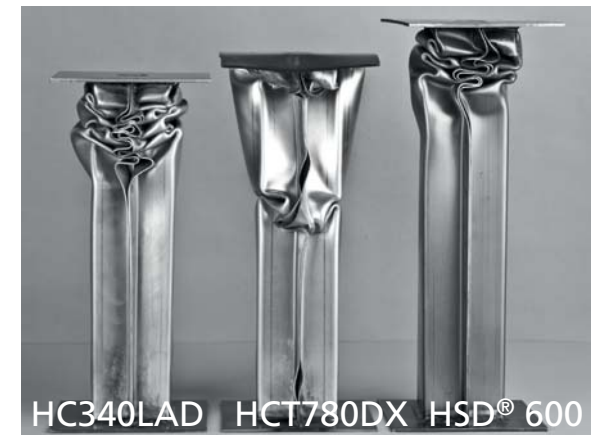
Crush testing under the same load with the same sheet thickness
