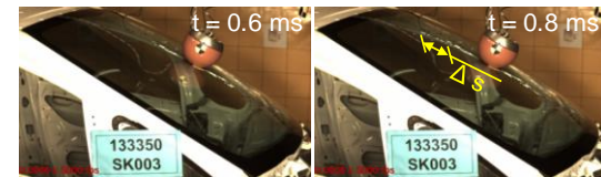
Crack propagation during impactor test ( v = \Delta s / \Delta t \approx 150 mm / 0,2 ms = 750 m/s)
