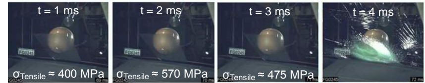
Chronological sequence of impactor test (picture from [RIE05], stresses from internal simulations)
