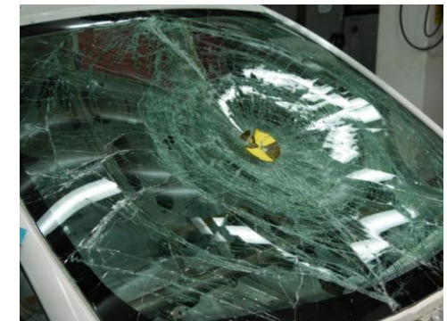
Fracture pattern after test
