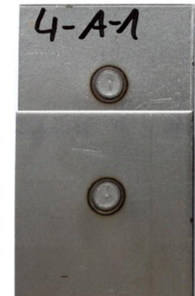
interfacial fracture mode
