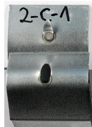
nugget pullout fracture mode
