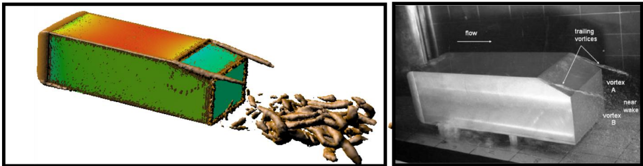
Figure 9 Q criterion visualization in the wake of the body next to a picture from the experiment by [5]
