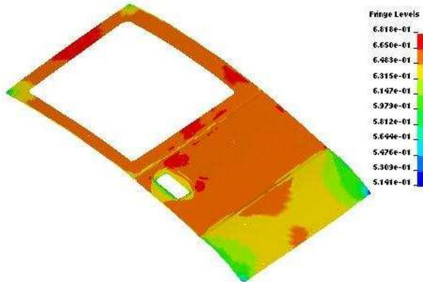
Springback amount (mm) in Z is shown in the figure below.
