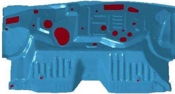
*Trimmed-out Holes Filled with LS-PrePost*
