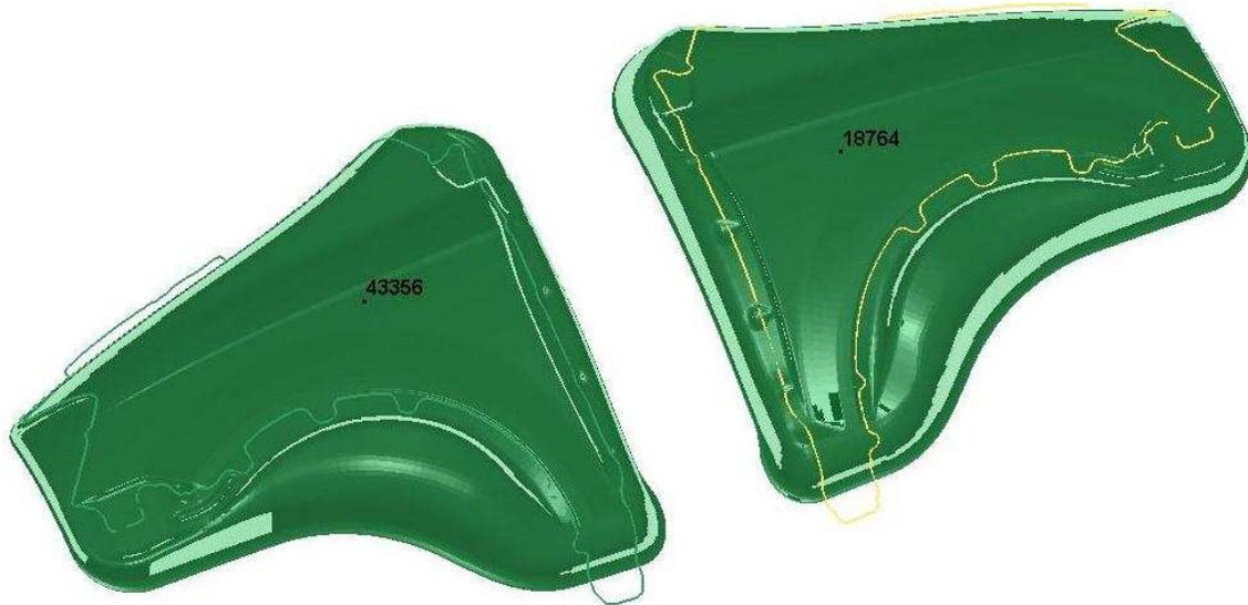
*Using the two nodes from the stationary tools at its home position to define NSEED1 and NSEED2 for trimming of a double-attached part (NUMISHEET2002 Fender Outer)*
