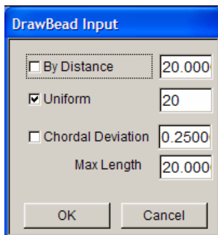
Figure 9.4.9 Define the density of points on the drawbead line
